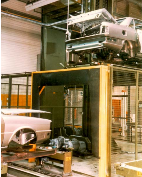
Fig. 48.1 Vertical conveyor for car bodies Pole-changing motor in the ratio 1:6; with spring-loaded brake and (covered) square shaft end for setting up; reserve drive ready
