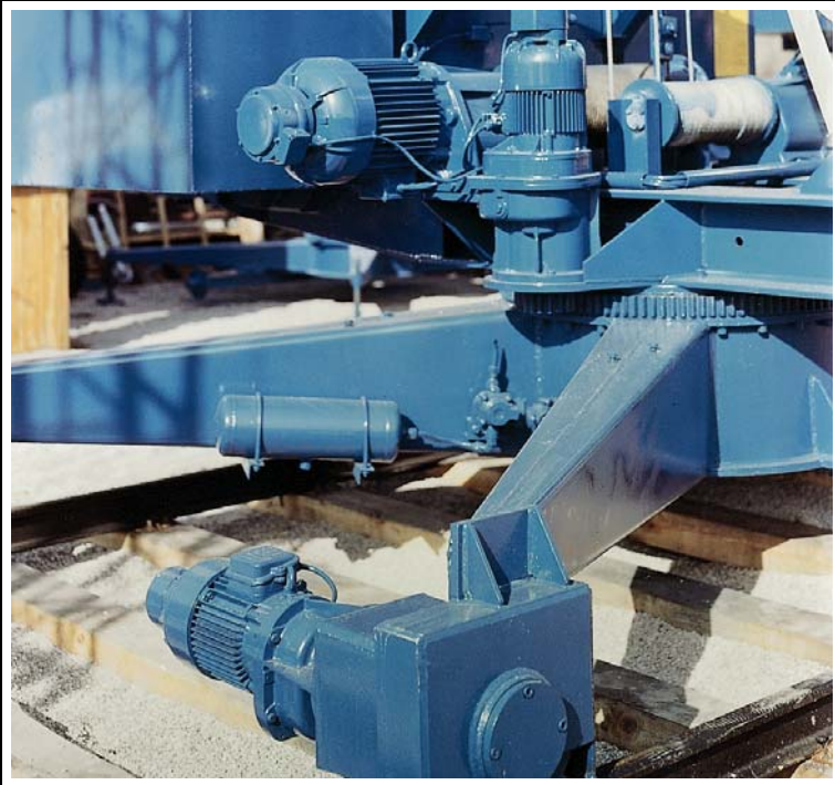
Fig. 14.4 Special DL-type cage motors on the slewing gear and travelling gear of a tower slewing crane
