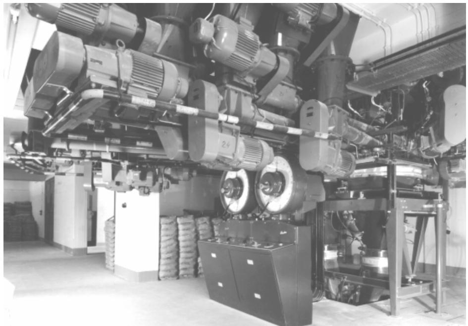
Fig. 44.3 Metering screws for filling and fine feed; friction brakes with a short overtravel time prevent unwanted overfilling
