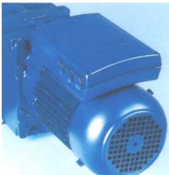
Fig. 54.4 "Eta-K" Three-phase geared motor with built-on frequency inverter to form a compact drive Rated outputs P_N to 7.5 kW Integrated protective devices against overload, overcurrent, phase failure, overvoltage and undervoltage. Thermal monitoring for the motor and inverter. Connected by a plug to the motor unit Degree of protection IP65.
