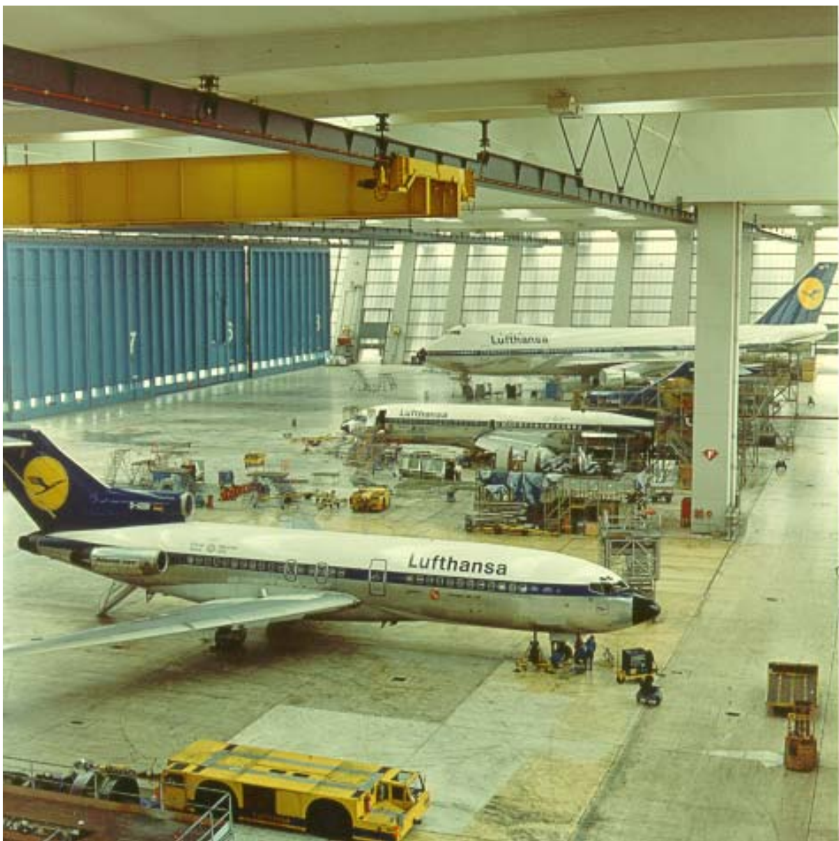
Fig. 2.4.4 Overhead travelling crane used to service passenger aircraft. Particular requirements on soft starting and stopping of the crane's travelling gear
