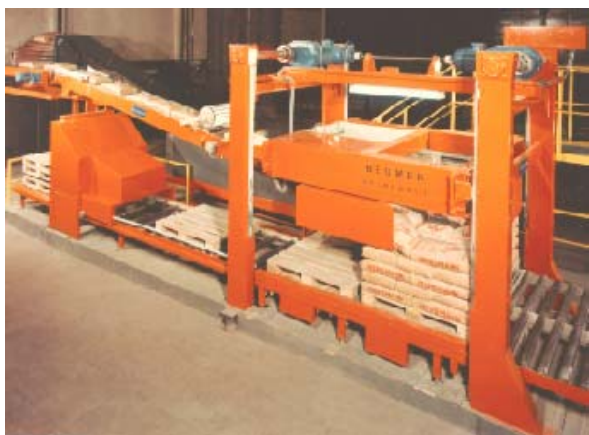
Fig. 48.3 Palleting machine for cement sacks Bevel-gear motor with controlled synchronization of the four drive units; pole-changing 1:6
