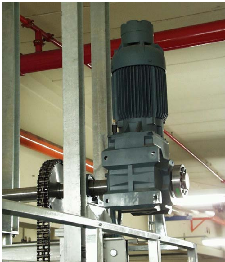
Fig. 19.2 Hoist drive in the automotive industry, driven by a geared motor. Shaft-mounted bevel gear When descending, the motor is driven at hyper-synchronous speed, generating power back to the mains
