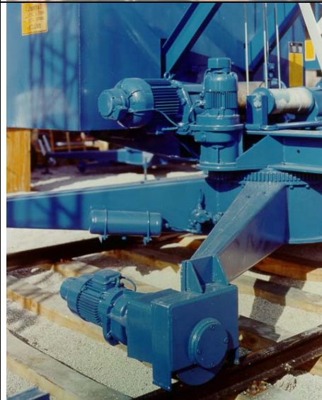
Fig. 32.3 Geared brake motors on the lifting gear, slewing gear and travelling gear of a tower slewing crane Possible applications of geared brake motors
