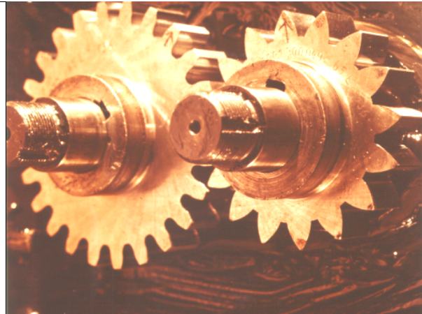
Fig. 10.3.4 Test gear wheels in the FZG test rig for testing the high-pressure properties of lubricants in extreme conditions due to poor tooth form
