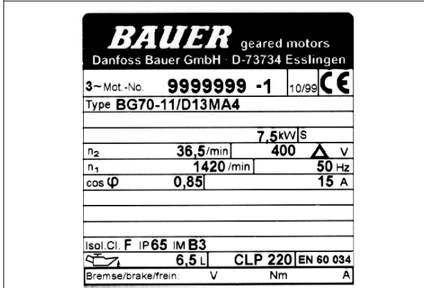
Fig. 10.3.7 Example of currently used information on the main plate with internationally understandable abbreviations
