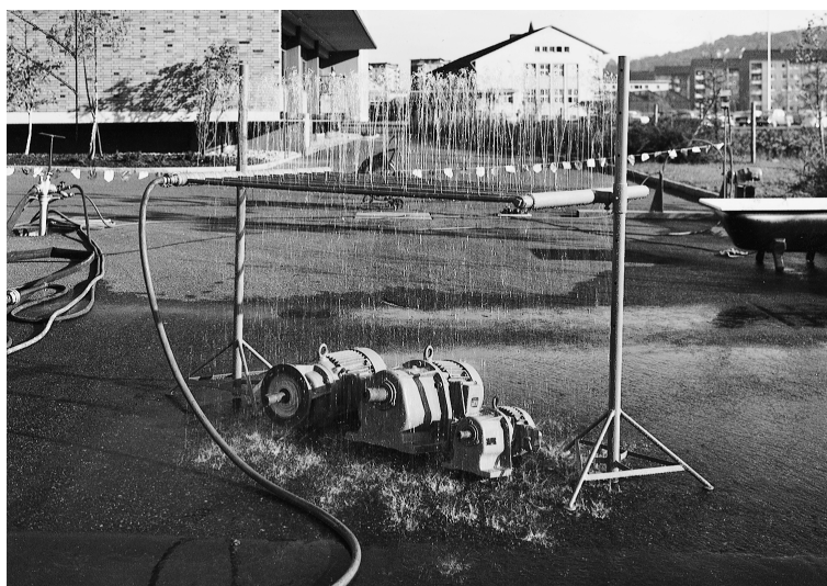
Fig. 4.7.1.2 Long-term exposure of geared motors to rain to test fitness for outdoor installation
