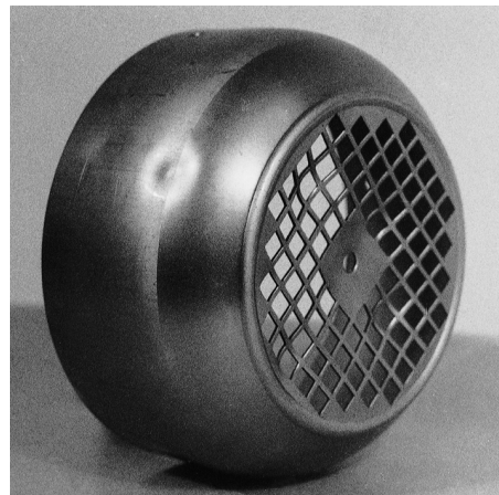
Fig 4.8.1.3 Reinforced fan cowl after the impact test
