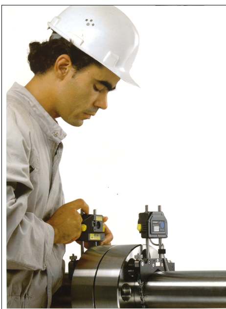
Fig. 7.3.3 Aligning the shafts using a laser and computer (Source: ROTALIGN Prüftechnik AG, Ismaning)
