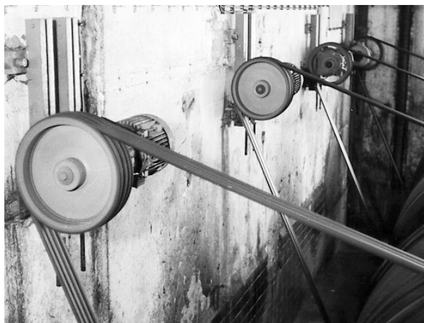
Fig. 8.7.1 Example of calculation the overloading by overhung load on the output shaft without indication via current reading
