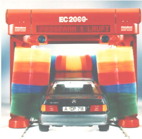
Fig. 4.4.5 Special protective measures are recommended for electrical equipment located in the area directly affected by the water from a car wash.
