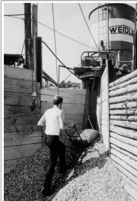
Fig. 5.1.2.1 Digger as an example an electric motor with a varying load during a working cycle
